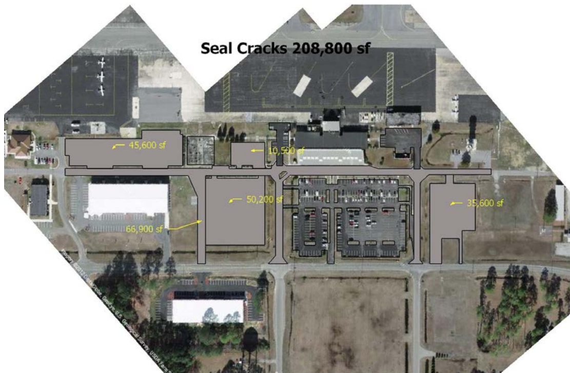
Figure G-1: NCGTP parking areas in need of preventative maintenance.
